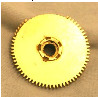
Waterbury main wheel damaged by the sudden uncoiling of a fractured mainspring
