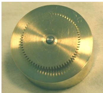
New main wheel attached to reconditioned barrel.
